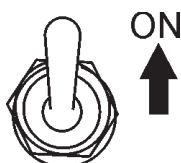
Figure 19. Idle Control Switch (ON)
