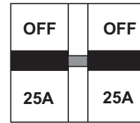
Figure 25. Main Circuit Breaker (OFF)
