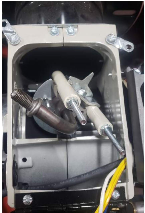
5. Remove nozzle line assembly from burner, being careful not to damage the electrodes or insulators while handling. To ease removal of the assembly rotate assembly 180° from installed position after pulling partially out of tube.
