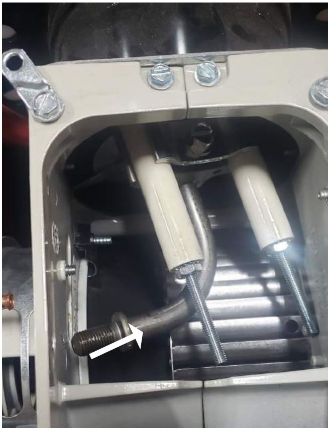
5. Remove nozzle line assembly from burner, being careful not to damage the electrodes or insulators while handling. To ease removal of the assembly rotate assembly 180° from installed position after pulling partially out of tube.
