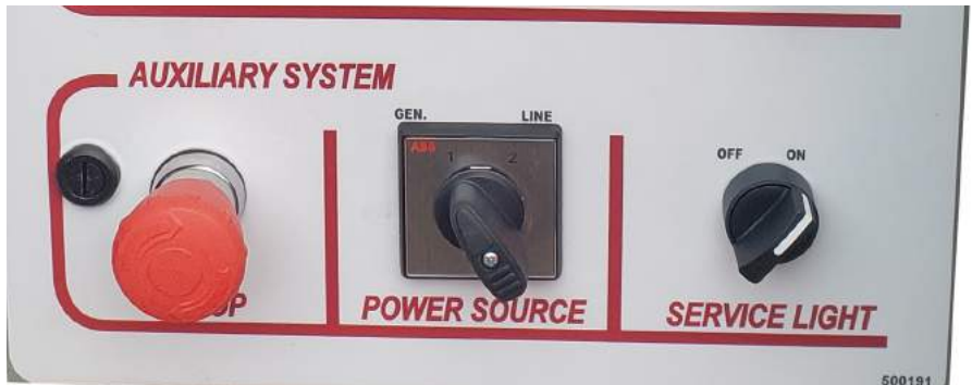
Power Source Selector Switch
